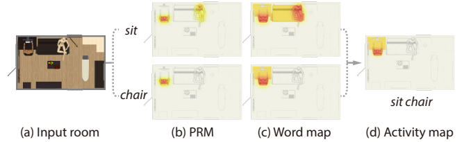
Fig. 5. Creation of an activity map: we combine the PRM for a word with an object mask to obtain the word map, and intersect the two word maps to obtain the activity map for a verb-noun label. The position probabilities of the word and activity maps are shown as heat maps ranging from white (minimum) through yellow and up to red (maximum value).
